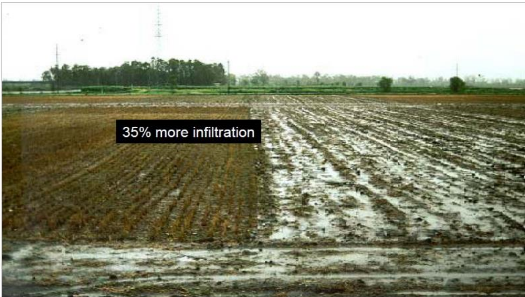
Figure 24b: A dramatic demonstration of the impact of soil compaction. The soil of an experimental plot (Italy) has been subjected to heavier loads on the right hand side of the image than on the left hand side. The compacted structure of soil on the right has resulted in a reduced infiltration capacity of the soil leading to surface ponding and waterlogging. © Ezio Rusco;
